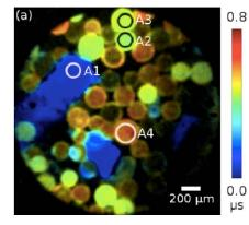
Image (a): Lifetime images of beads infused with different Ir compounds and fluorescent plastic acquired with TimepixCam, a previous model of the TPX3Cam.
