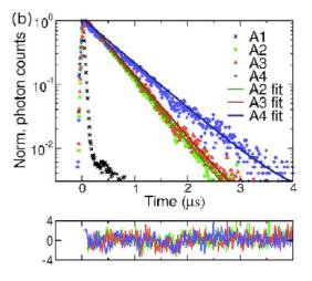
Image (b): Intensity as a function of time (phosphorescence decays) for areas A1-A4 indicated in (a), with monoexponential fits to the phosphorescence decays and residuals of the fits.
