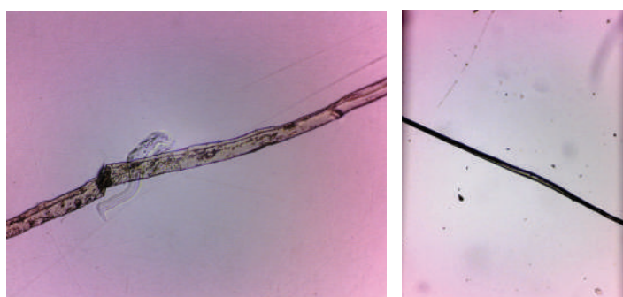
Polyethylene terephthalate (PET) single fiber top left – video micrograph of fiber in compression cell. Top right - video micrograph of fiber viewed through the ATR crystal. Bottom – IR spectra in transmission and ATR modes.
